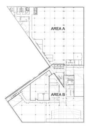
The MEP systems in this building are extensive so the rough-in construction sequence will take detailed coordination to plan and execute. Rough-in work will take place in the standard sequence of ductwork first, plumbing piping next, finishing with mechanical piping, electrical
